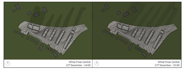
Figure A.9 – Overshadowing Image on December 21st at 2 p.m. and 3 p.m.
