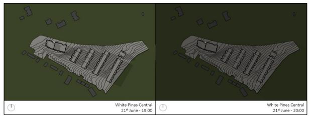
Figure A.6 – Overshadowing Image on June 21st at 7 p.m. and 8 p.m.
