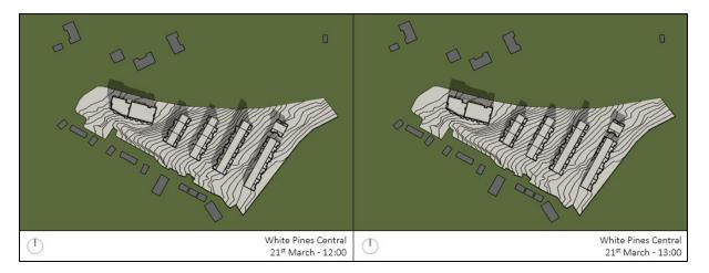
Figure 27 – Overshadowing Image on March 21st at 12 p.m. and 1 p.m.
